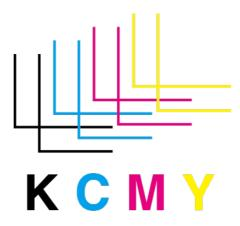
Trim Marks use registration colour to check for misalignment during printing. If any of the printing plates are misaligned, the colour ink will show which one, and we can make adjustments to re-align them.
